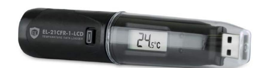
This standalone data logger measures and stores more than 16,000 temperature readings over a -35 to +80°C (-31 to +176°F) range with a resolution of  $0.5^{\circ}$ C (1°F).
