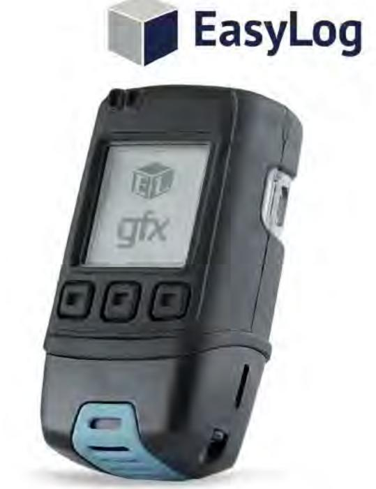
This stand-alone data logger measures and stores over 250,000 temperature and humidity readings over a -30 to +80°C (-22 to +176°F) and 0 to 100%RH range at a resolution of 0.1°C (0.2°F) and 0.1%RH.
