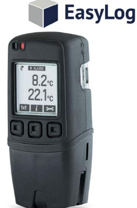
This standalone data logger measures and stores more than 250,000 temperature readings from two K, J or T-type thermocouple probes at a resolution of 0.1°C (0.2°F). It comes supplied with two K-type thermocouples capable of measuring from 0 to 200°C (32 to 392°F).
