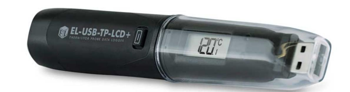
This standalone data logger measures and stores more than 32,000 temperature readings over a -40 to +125°C (-40 to +257°F) range and is supplied with a high accuracy thermistor probe. See page 4 for more details.
