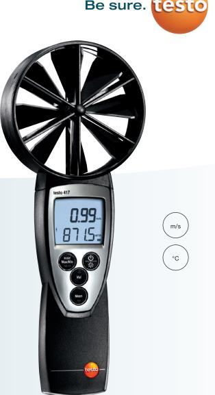
testo 417 is a compact, large-area anemometer with a built-in flow velocity / temperature vane. It measures flow velocity, volume flow and temperature. Thanks to the integrated measurement with the 100 mm vane, it is ideally suited for measurements at air input and output vents. The flow direction, i.e. blowing or sucking flow, is visible in the display. The optimum funnel set additionally allows measurements on ventilation grilles and disc outlets.
