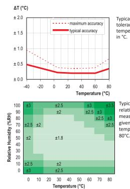
Typical and maximal tolerance for temperature sensor
