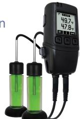
This standalone data logger measures and stores over 250,000 temperature readings over a -40 to +125°C (-40 to +257°F) range at a resolution of 0.1°C (0.2°F).
