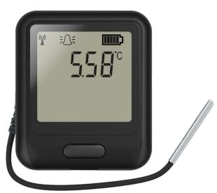
The EL-WiFi-21CFR-TP+ has a protection rating of IP42 and the probe IP67. The unit is freestanding, but it can be attached to a wall or surface using the bracket provided. The unit can be clipped in and out of the bracket as required.
